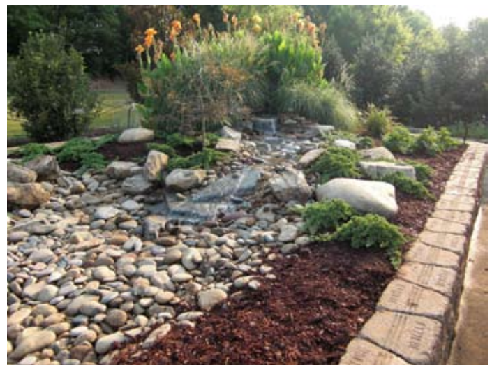
A pondless water feature was added to Prattville’s Butch Ray Fragrance Garden at Overlook Memorial Park. Designed to “disappear” through a stack of native rocks, the water is then collected into a sump below the rocks and recycled back through the feature, keeping the water cleaner, clearer and preventing “pond scum” from developing. Such water features are much more child-safe than traditional ponds since there’s no pooling of water, virtually eliminating any drowning risk. In addition, the issue of mosquito breeding is alleviated because this feature will not generate stagnant water. Photo by City of Prattville horticulture employee Matthew Morgan.
